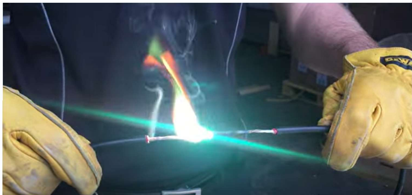
Illustration: DC Solar Array - Arc fault demonstration
