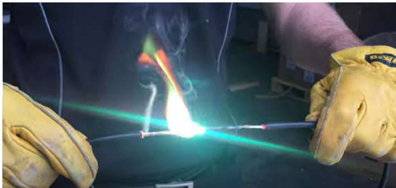
Illustration: DC Solar Array - Arc fault demonstration
